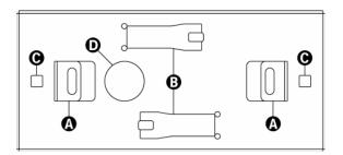
**WARNING:** insert the gasket in the hole through which the cables pass, as shown in the picture. Pierce the gasket in order to let pass the cables to be connected to the central unit, being careful of narrowing them in order to avoid the entrance of bugs and small animals.
