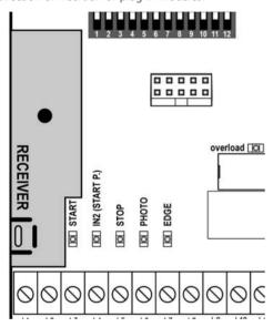
The MR1 receiver module has 4 channels, each with an associated command on the **City7** control unit:
