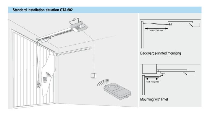
The charts shown above illustrate a possible installation situation for GTA 602. As illustrated, the operator is also suitable for backwards-shifted mounting and mounting with lintel. For these special cases, special door brackets are required. Please have a look at our accessories listed as Z1.
