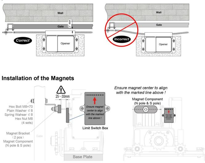
Before install limit switch, make sure the gate opener is put in manual operation. (the clutch connected with gear shaft is disengaged) and the mains power supply is disconnected. Position the two Magnet Components approximately on the gate and move the gate by hand to fix them in place.
