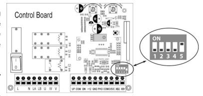
NOTE: The midway mode function would be disabled if both DIP switches are turned off. Factory default setting is disabled. The midway mode could be activated by pressing button B of the remote control when the gate is in the full closed position.
