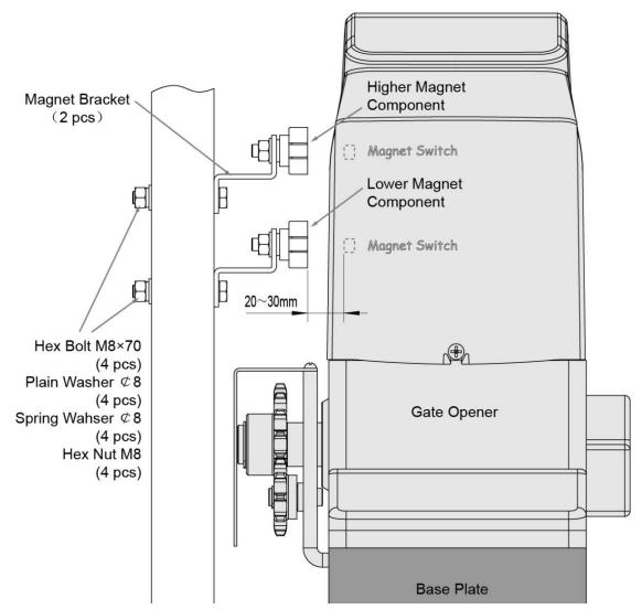
Before install limit switch, make sure the gate opener is put in manual operation. (the clutch connected with gear shaft is disengaged) and the mains power supply is disconnected.
