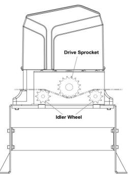
6). The chain brackets must be mounted to the same height as the chain on the idler wheels.
