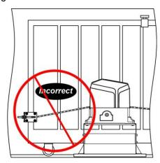
7). Make sure there is 1" distance at least between the wheel cover and the gate after you position the base plate.
