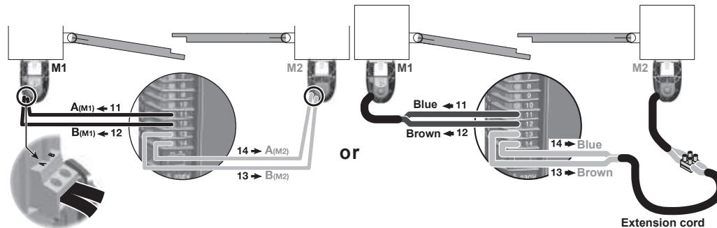
The motor M1 moves the left leaf, which opens first and closes last:
