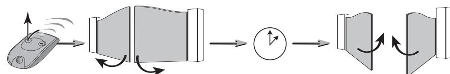
It is possible to maintain the gate in the open position by giving a short press order on remote control key during temporisation
