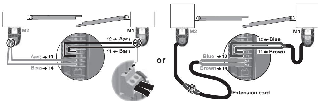
The motor M1 moves the right leaf, which opens first and closes last:
