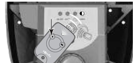
**!** At the end of the memorization cycle, only the PROG and ON/OFF lights are lit, the electronics waiting for memorization of leaf displacement
