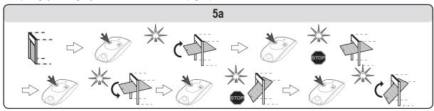
Partial opening cycle using Keytis or similar remote controls (Fig. 5b)
