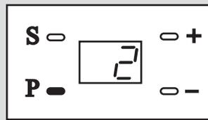
5. If the door has moved downwards to the required position, press "P" to save the lower end point.
