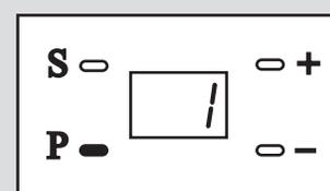
6. If the door has moved upwards to the required position, press "P" to save the upper end point.
