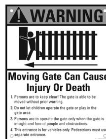
Install warning decals, one on each side of gate operator
