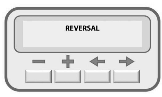
To disable the rollback just press the (-) key to enable press the (+) key.
