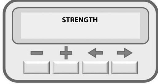
The force leaves the factory at the maximum level, to decrease it just press the (-) key to the desired level, to increase it just press the (+) key.
