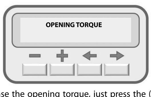
To increase the opening torque, just press the (+) key to the desired torque level and to decrease it, just press the (-) key.
