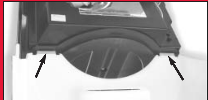
FIG. 10-1 Slide hinges into motor cover.
