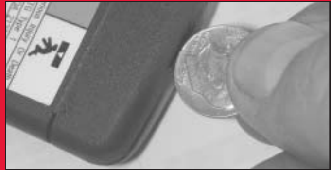
FIG. 9-1 Open battery cover.
