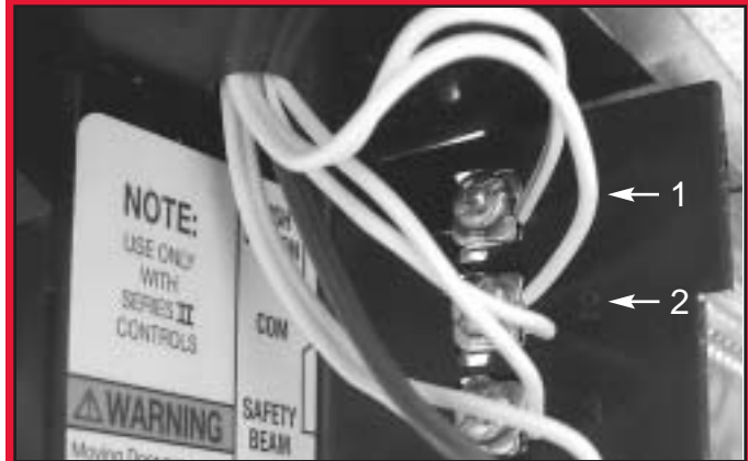
FIG. 5-1 Terminal attachments at power head.
