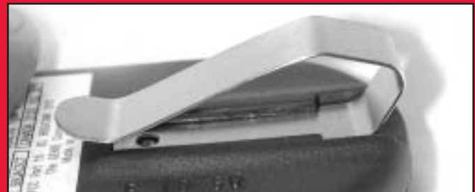
FIG. 9-3 Attach visor clip.
