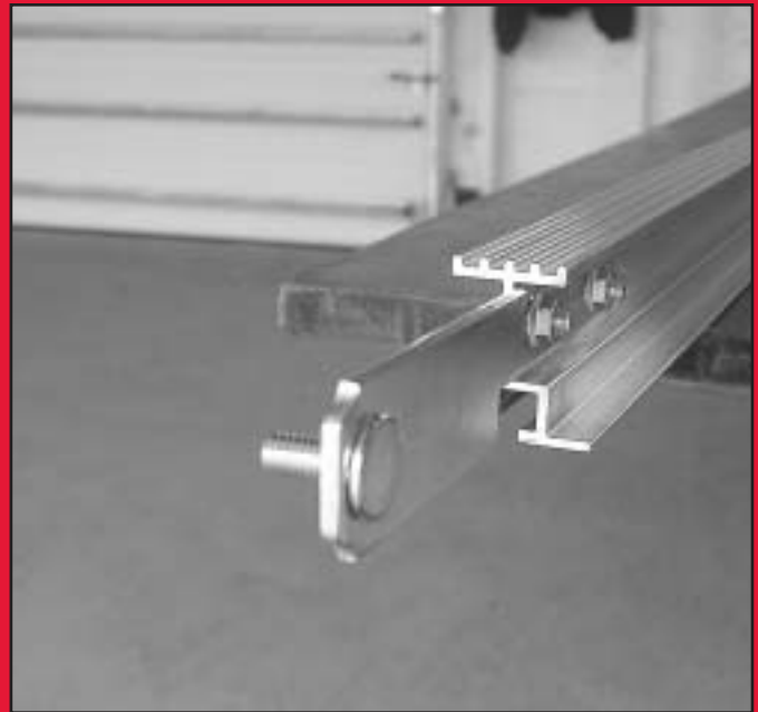
FIG. 1-1 Attach boom strap.
