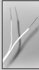
FIG. 3-6 Splitting and stripping.
