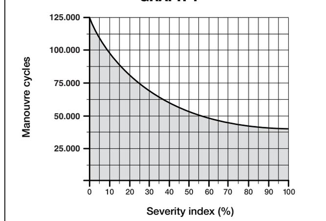
Example of durability calculation: automation of a gate with a leaf length of 1.5 m with weight of 220 kg, for example, in a location subject to strong winds. Table 1 states the "severity index" values for this type of installation: 10% ("Leaf length"), 25% ("Leaf weight") e 15% ("Installation in windy areas").
