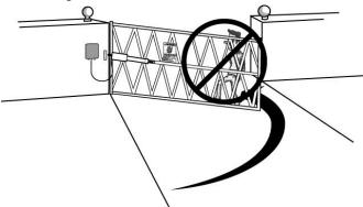
8. Pedestrians should never cross the pathway of a moving gate. The gate opener is not acceptable for
