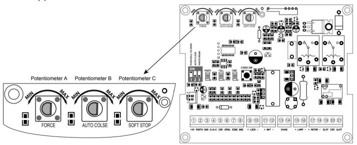
**Potentiometer A** is used to adjust the stall force the gate opener. Turn the potentiometer clockwise to increase the stall force, and turn it counter-clockwise to decrease the stall force.
