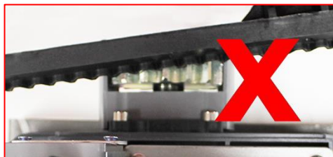
Gear rack misaligned. Do not attempt to use if misaligned.
