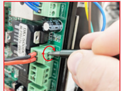
Tighten with a screwdriver to secure the wire in place.
