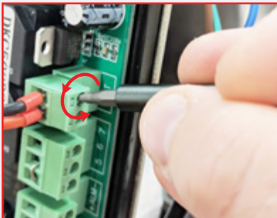
Using a screwdriver, loosen the screw on the side of the terminal.
