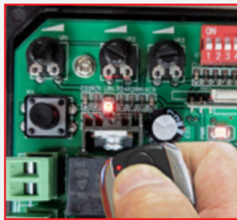
While the light is on, press the first button on the remote control twice.
