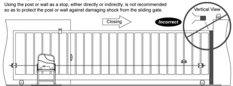
In sake of safety, a positive stop must be mounted on the two end of ground track.
