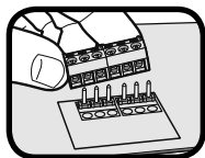
Terminal blocks can be removed to simplify wiring.
