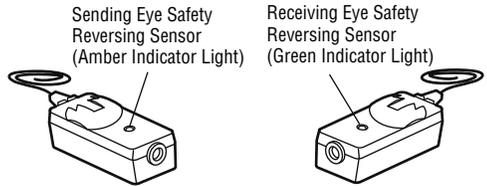
**3. My door reverses for no apparent reason:** Repeat safety reverse test after adjustments to force or travel limits. The need for occasional adjustment for the force and limit settings is normal. Weather conditions in particular can affect door travel.
