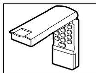
3. Release the button when the motor unit lights blink. It has learned the code. If light bulbs are not installed, two clicks will be heard.
