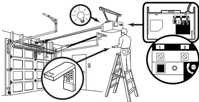
1. Press and release the “learn” button on motor unit. The learn indicator light will glow steadily for 30 seconds.
