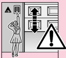
**Permanently installed controls (such as buttons or similar devices) should be installed within sight of the door but well away from any moving parts and at a height of at least 1.5 metres. It is vital that they are installed out of the reach of children!**
