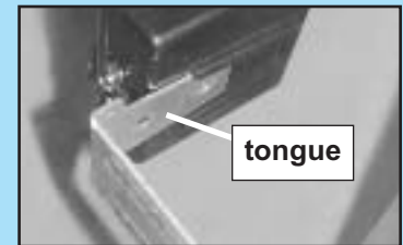
FIG. 3-3 Attaching STB's to brackets.
