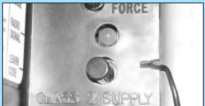
FIG. 8-1 Learn code button and LED
