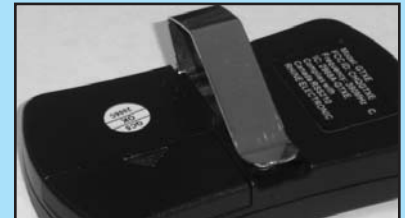
FIG. 8-2 Match battery polarity.
