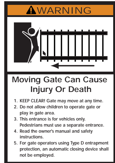
warning label (1) installed on operator housing
