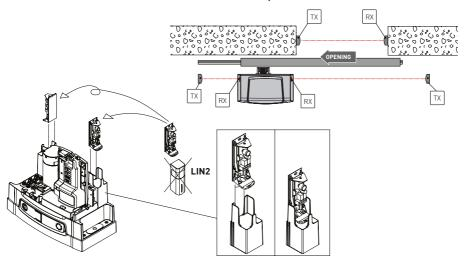
Additional photocells can be installed inside the gearmotor casing of Ditec NEOS, to protect both opening and closing movements by using the LIN2 photocell.
