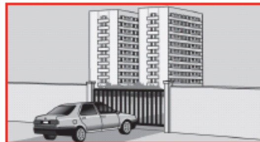
Class II (Commercial/General Access Vehicular Gate Operator) - A vehicular gate operator (opener or system) intended for use in a commercial location or building such as a multi-family housing unit (five or more single family units), hotel, garages, retail store, or other buildings servicing the general public.
