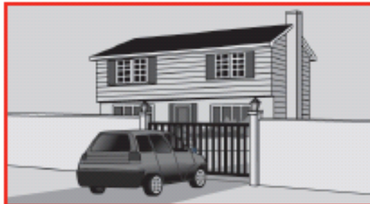
Class I (Residential Vehicular Gate Operator) - A vehicular gate operator (opener or system) intended for use in a home of one to four single family dwellings, or a garage or parking area associated therewith.
