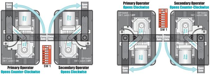
Drive motors face the same direction in a dual gate installation.
