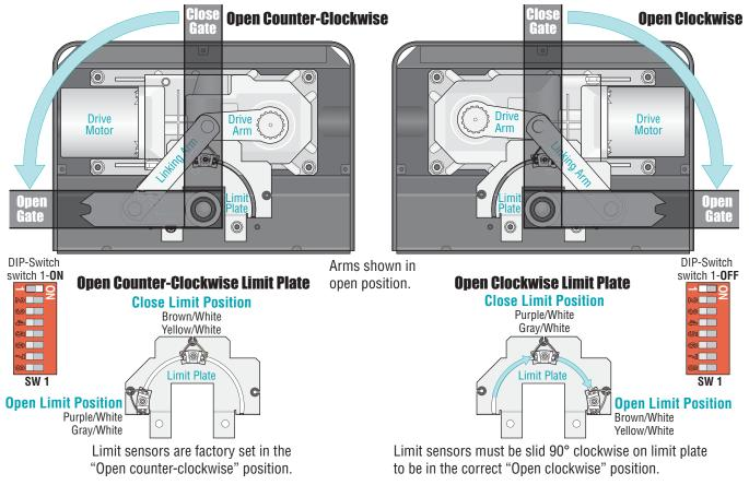
Note: Final limit adjustments will be made after AC power has been connected.
