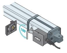
Use key to unlock and remove the cover. Remove allen wrench from inside of cover.
