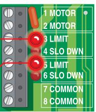
Note: 3 and 5 limit LEDs can be Open or Close limits according to SW 1, switch 1 and 2 settings.
