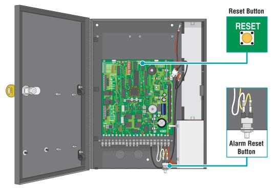
Once the gate has been reset, an open or close command is needed to start the gate operator. Most activating commands will cause the gate operator to cycle to the open position. This includes activation of a key switch or open command and activation of an open loop. Activation of a close command will run the gate to the closed position.
