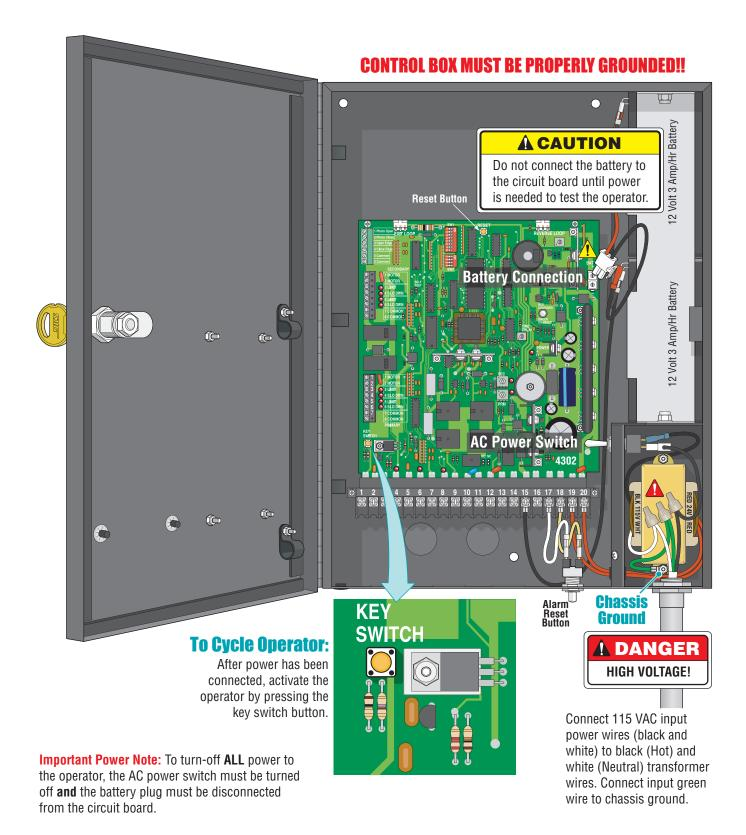
It is recommended that a surge suppressor be installed on the high voltage power lines.
