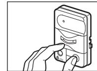
3. Continue holding both buttons while you press the push bar on the Motion Detecting Control Console (all three buttons are held).
