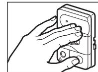
4. Release buttons when the motor unit lights blink. It has learned the code. If light bulbs are not installed, two clicks will be heard.
