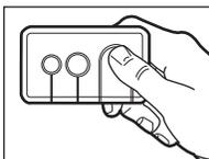
3. Release the button when the motor unit lights blink. It has learned the code. If light bulbs are not installed, two clicks will be heard.
