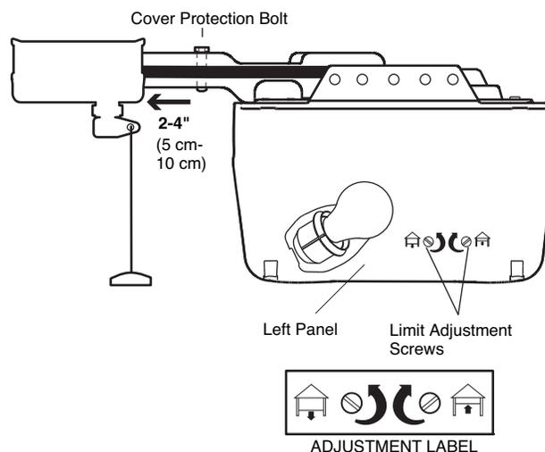
Test the door for binding: Pull the emergency release handle. Manually open and close the door. If the door is binding or unbalanced, call for a trained door systems technician. If the door is balanced and not binding, adjust the DOWN (close) force. See Adjustment Step 2.
