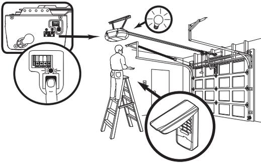
1. Press and release the "learn" button on motor unit. The learn indicator light will glow steadily for 30 seconds.
