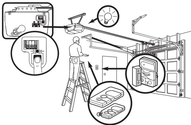
1. Press and release the "learn" button on the motor unit. The learn indicator light will glow steadily for 30 seconds.
