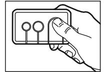
2. While holding the remote button, press and hold the LIGHT button on the door control.
