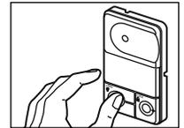
3. Continue holding both buttons while you press the push bar on the door control (all three buttons are held).
