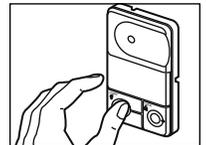
3. Continue holding the ENTER and LIGHT buttons while you press the push bar on the door control (all three buttons are held).
