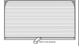
This test should be repeated monthly to ensure the safe operation of your opener.
