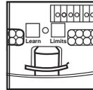
Orange LED will turn off and courtesy LEDs will flash once
