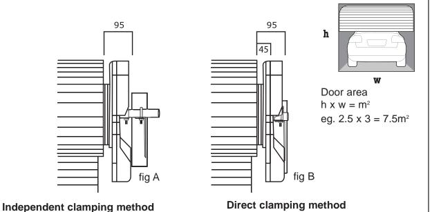
Ensure that there is at least 45mm from the edge of the curtain to the edge of the bracket. If the roller door drum is on the edge of the curtain or is a smaller diameter, additional clearance may be required.
