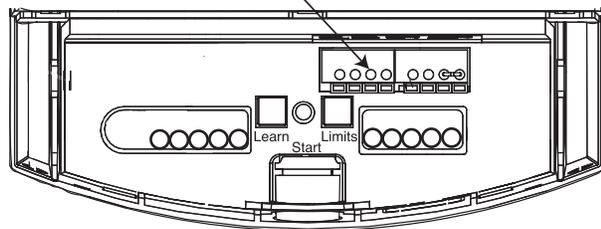
**Remove cover: Push cover plate up, then lever out from the button.**
