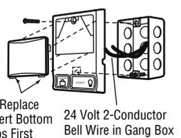
**Figure 3** MULTI-FUNCTION DOOR CONTROL (BACK)
