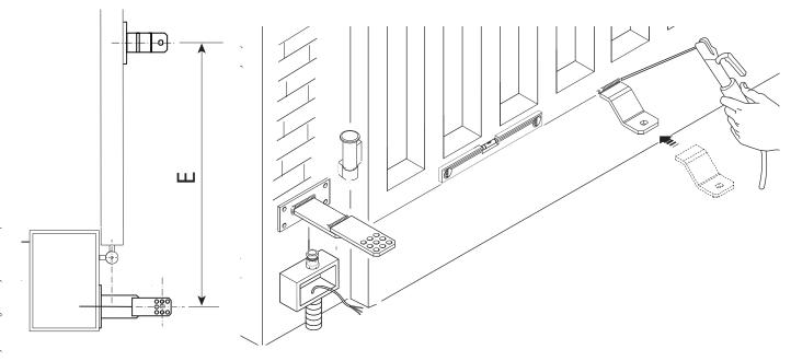
Fasten the gearmotor to the braces by using the supplied nuts and bolts.
