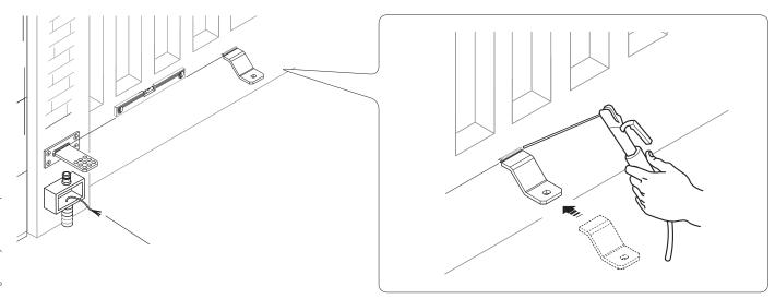
$\square$  On non-metallic leaves, assemble and weld the two parts of the brace - use suitable screws to fasten.
