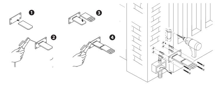
Open the gate to 90°, weld or fasten the gate brace using suitable bolts (while respecting quota E as shown in the table).
