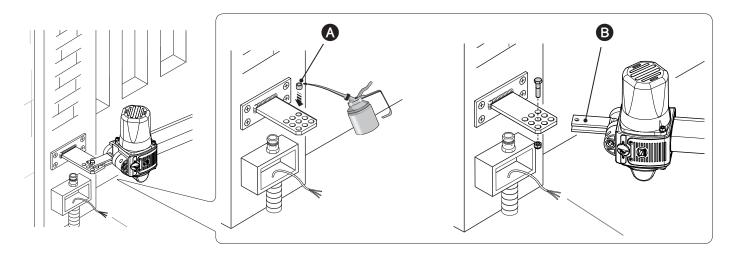
Open the leaf, fit the pinion into the gate brace and fasten it using the supplied washer and nut.
