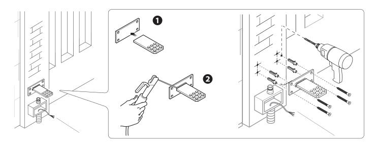
Weld the gate brace to the leaf following the measurements shown on the table.
