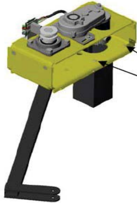
Figure 7: Installation of drive unit to mounting bracket
