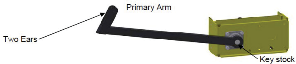
Figure 6: Connecting the primary arm to the operator chassis
