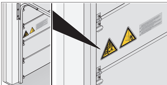
Fig. 1.2 Sticker on door panel
