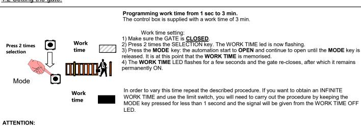
EVERY TIME THAT THE CONTROL UNIT IS TURNED ON THE WORKING TIME IS RELOADED. THE FIRST STEP BY STEP COMMAND IS ALWAYS OPEN EXCHEPT WHEN THE OPEN LIMIT SWITCH (IF PRESENT) IS ACTIVATED.
