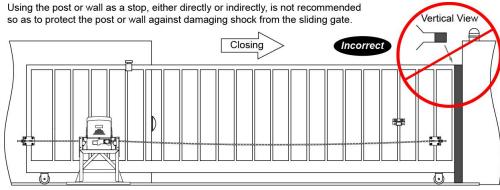
In sake of safety, a positive stop must be mounted on the two end of ground track.
