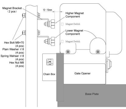
with the motor. *The magnet should be 20-30mm away from the magnetic limit switch.* If it is too far away, the switch will fail to work. The distance between the magnet and the opener should be 10-15mm with the opener cover on. Adjust the position of the magnet until the positions of the opening and closing meet the requirement.
