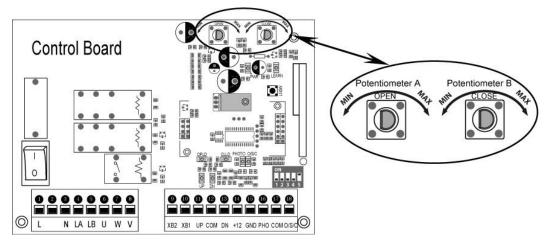
WARNING: Photocell must be installed with the gate opener as entrapment protection for safety when you set stall force to maximum.
