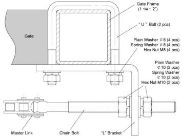
chain bolt to the L bracket and fix them each other by washers and nuts temporarily. (Nuts will be further adjusted for a proper chain tension later)
