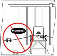
2). The opener must be parallel to the gate.
